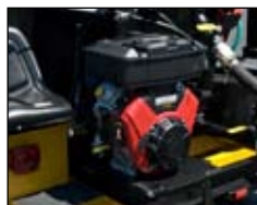
16 HP twin cylinder gas engine powers the system
