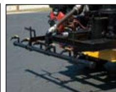
Optional distributor bar to apply up to a 16 foot pass
