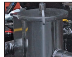
2.5 gallon material filter for extended spray periods
